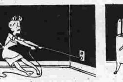
4. Handle your cord with care. Pull the plug, not the cord, and, above all, don't let the cord get damp. When you push plug in, be sure the switch is "OFF" and al
